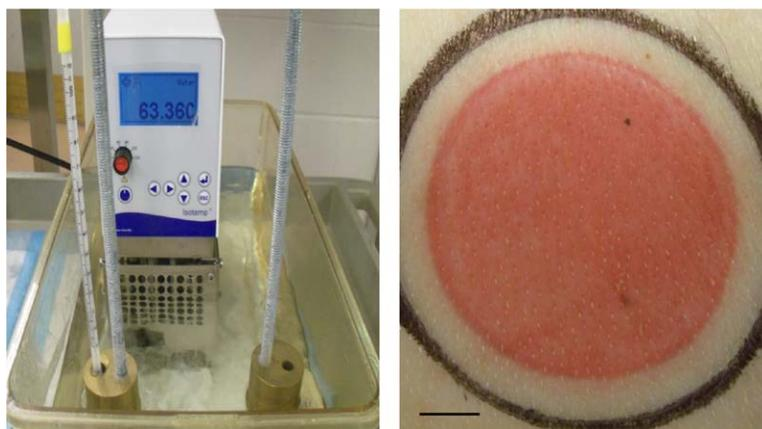
**Figure 1.** Left panel: Photograph of temperature-controlled water bath containing two 2.1 kg brass cylinders with an area of 12 cm<sup>2</sup> at each end. Each cylinder contains openings for insertion of thermometers to confirm block temperature. Right panel: Photograph of a representative contact burn produced by contact with heated brass cylinders. Scale bar: 1 cm.
